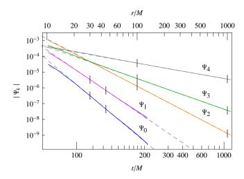
FIG. 2. The falloff of the Weyl scalars along the approximate null geodesic  $\lambda_1$  corresponding to the first inspiral peak of  $|\Psi_4|$  on the x-axis. The falloff rates obtained from fitting in the intervals indicated by vertical black lines are indicated in Table III.
