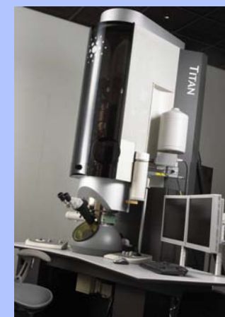
FEI Titan 80-300 aberration corrected TEM.
