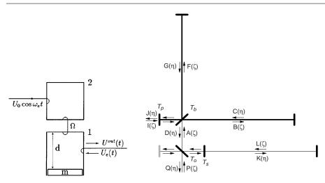
Fig. 1 Left: schematic diagram of the microwave speed meter on coupled cavities as given in [23,24]. Right: optical version of coupled cavities speed meter proposed in [21].
