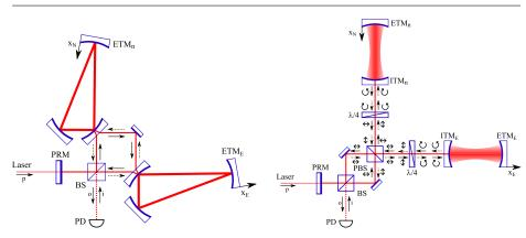
Fig. 2 Two possible optical realizations of zero area Sagnac speed meter. Left panel: The ring cavities can be used to spatially separate the ingoing fields from the outgoing ones, in order to redirect output light from one arm to another one [27]. Right panel: The same goal can be achieved idea is realized using optical circulator consisting of the polarization beamsplitter (PBS) and two  $\lambda/4$ -plates [28,29].
