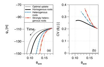
**Figure 3.** Model results of the simple model: (a) evolution of xylem potential over the course of root water uptake, (b) evolution of the coefficient of variation of soil water content during the simulation. Average initial soil water content is the same in all simulations. Only the unstressed uptake is shown. The time axis has been replaced by average volumetric soil water, which evolves parallel with time in this constant-flux experiment.
