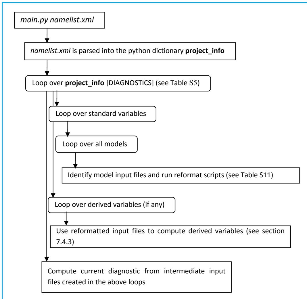
**Figure 2** ESMValTool control flow.
