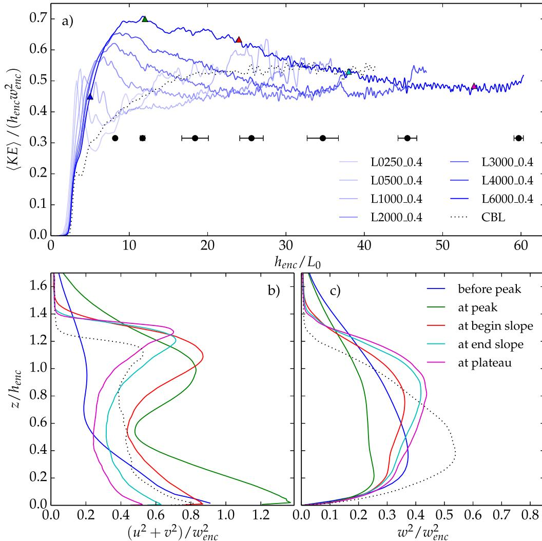
FIG. 6. (a) Time evolution of the vertically integrated KE for the cases with a flux in between the patches, described by parameter  $B_{0NP}/B_0 = 0.4$ . Five colored triangles on the graph of simulation L6000\_0.4 mark the time instants that correspond to the vertical profiles of (b) horizontal velocity variance and (c) vertical velocity variance. The dots in (a) mark the transition from the meso- to the microscale regime.
