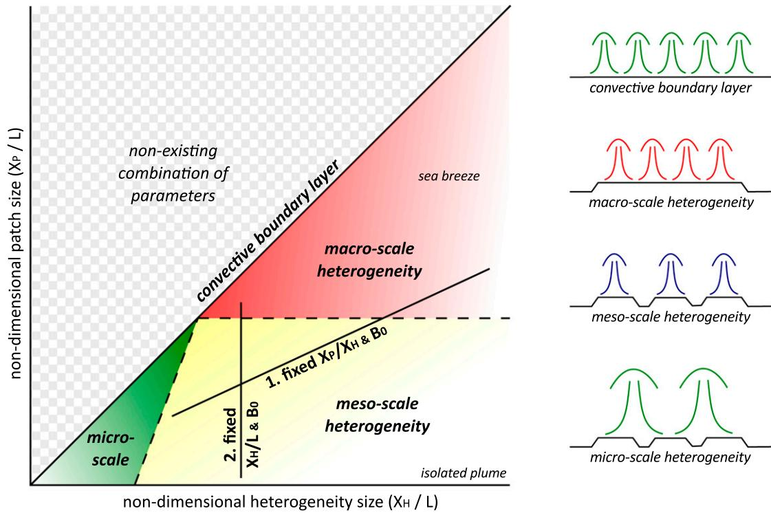
FIG. 2. Schematic view of the parameter space and the defined regimes. The two numbered thick lines represent the starting points of the simulations in the two experiments: The first diagonally through the parameter space at a constant patch size parameter  $X_P/X_H$ , and the second vertically at a constant heterogeneity size parameter  $X_H/L_0$ .
