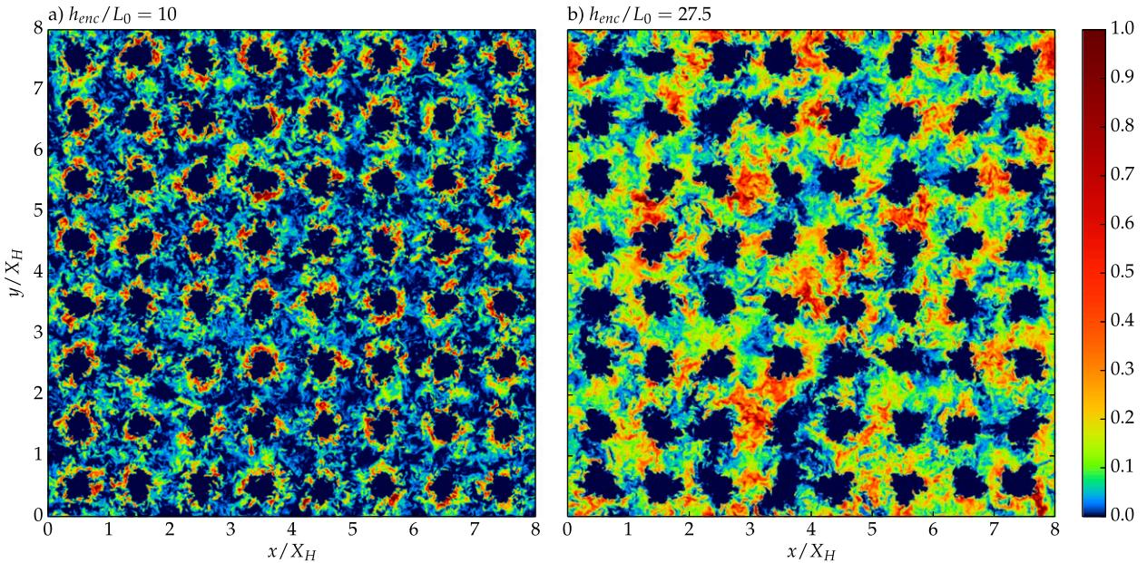
FIG. 9. Horizontal cross sections of the squared value of the downward velocity in simulation L1000\_0.0 at a height of  $4L_0$  taken at (a)  $h_{enc}/L_0 = 10$  and (b)  $h_{enc}/L_0 = 27.5$ . Both states have the same  $\langle KE \rangle_{(downdraft)} / (w_{enc}^2 h_{enc})$  (see Fig. 8), but the pattern is clearly different.
