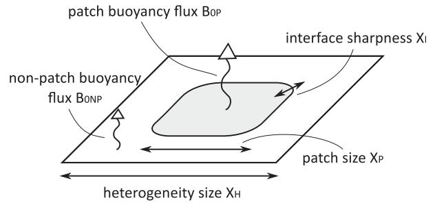
FIG. 1. Schematic view of a surface heterogeneity element. The surface of the physical model consists of an array of these elements in both horizontal directions.
