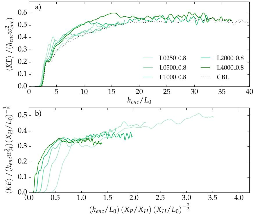
FIG. 14. Time evolutions of (a) the vertically integrated KE and (b) the scaled vertically integrated KE for the simulations from the first experiment with a  $B_{0L}/B_0$  of 0.8.
