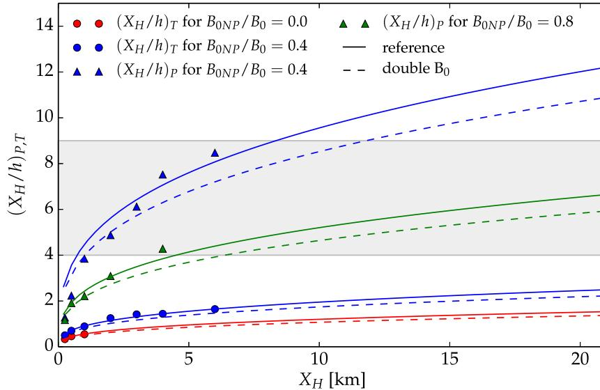
FIG. 15. The link between the absolute heterogeneity size and the ratio between  $X_H$  and  $h$  at which the transition occurs for the simulations in the first experiment. The colors correspond to those of the time evolutions in Figs. 5, 6, 11, 13, and 14. The gray shaded region marks the range that Patton et al. (2005) specified for the strongest secondary circulations.
