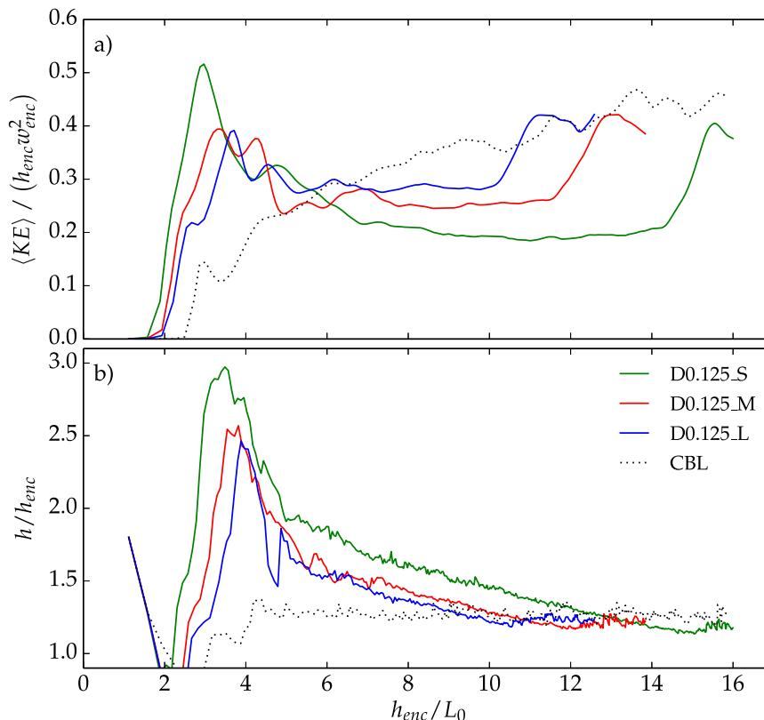
FIG. 7. Time evolutions of (a) the vertically integrated KE and (b) the boundary layer height for the DNS in the second experiment in which the patch size parameter  $X_P/X_H$  is varied.
