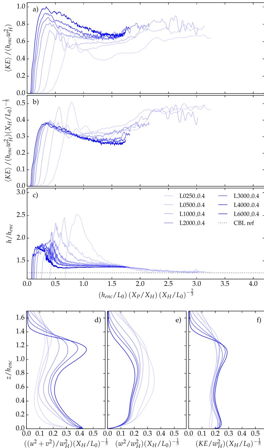
FIG. 13. Time evolutions of the scaled vertically integrated KE (a) without and (b) with correction factor applied and (c) CBL height. The vertical profiles of (d) horizontal velocity variance, (e) vertical velocity variance, and (f) turbulent kinetic energy taken for each simulation with a  $B_{0NP}/B_0$  ratio of 0.4 and at a scaled time value  $(h_{enc}/L_0)(X_P/X_H)(X_H/L_0)^{-2/3}$  of 0.75.
