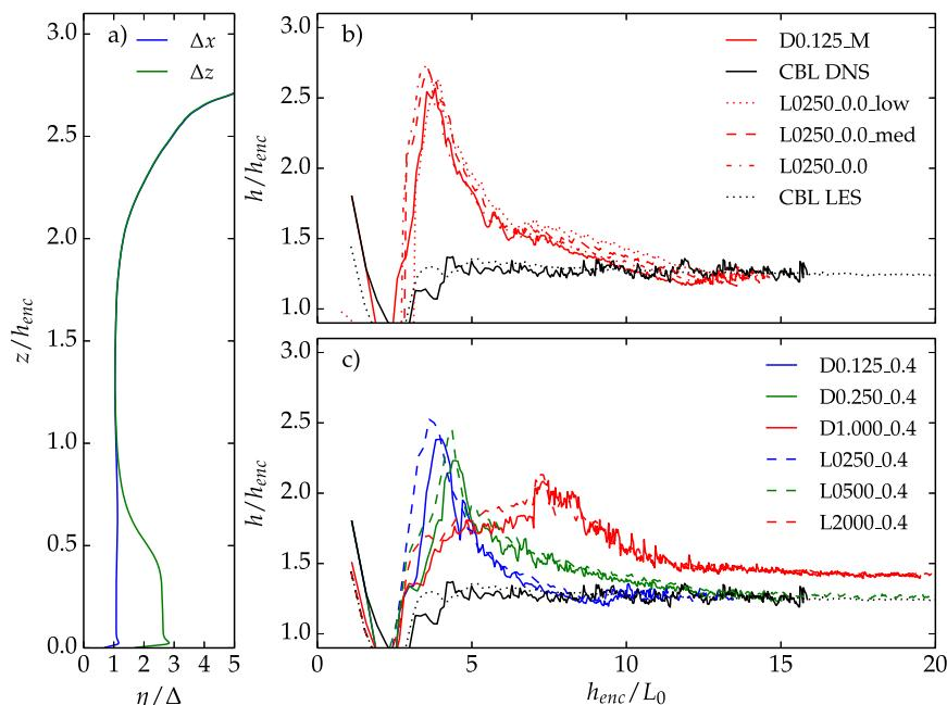
FIG. A1. (a) Ratio of the Kolmogorov length  $\eta$ , calculated following  $\eta \equiv (\nu^3/\epsilon)^{1/4}$ , to the horizontal ( $\Delta x$ ) and vertical ( $\Delta z$ ) grid spacing during the peak in KE in simulation D0.125\_M; time evolution of the scaled boundary layer height (b) for a resolution study for LES and (c) for a comparison of multiple cases between DNS and LES.
