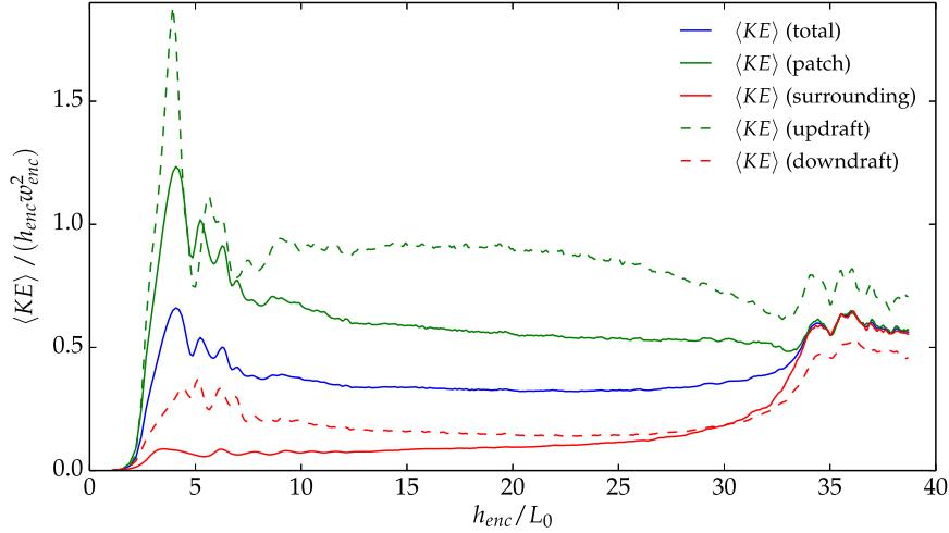
FIG. 8. Time evolution of the vertically integrated KE of case L1000\_0.0, corresponding to different sampling conditions.
