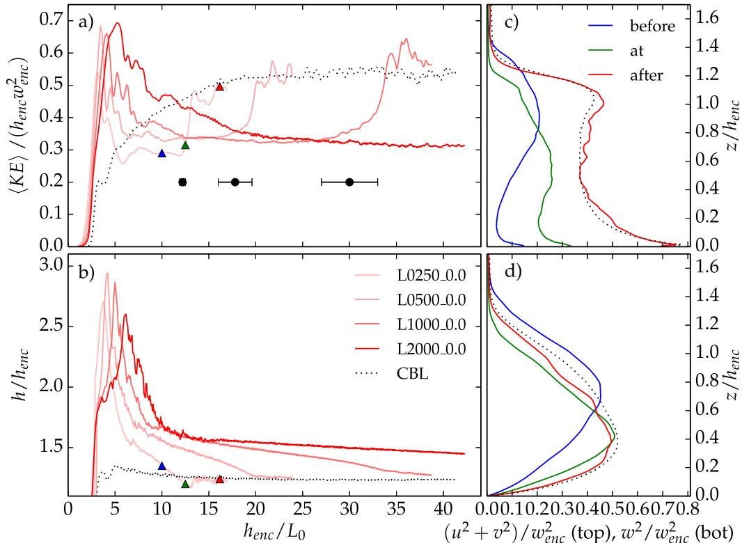
FIG. 5. Time evolutions of the (a) vertically integrated KE and (b) CBL height for simulations with  $B_{0NP} = 0$ . Three colored triangles on the graph of simulation L0250\_0.0 mark the moments that correspond to the three vertical profiles of (c) horizontal velocity variance and (d) vertical velocity variance. These triangles also mark the time instants at which cross sections in Figs. 3d–f are taken. The dots mark the transition from the meso- to the microscale regime.
