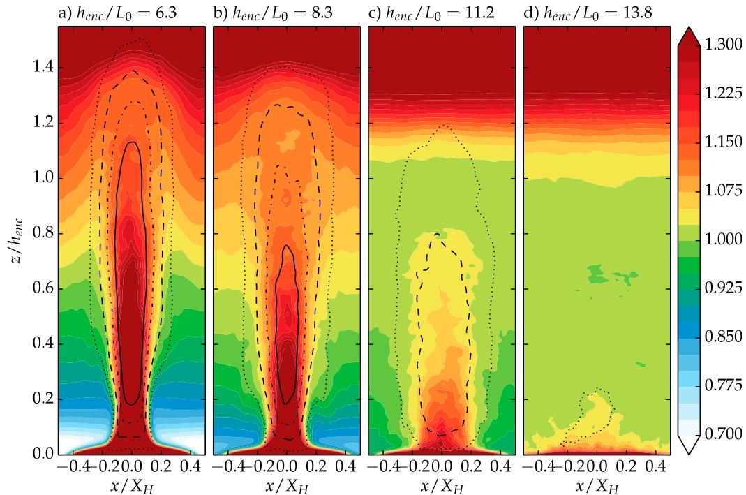
FIG. 4. Vertical cross sections of ensemble averages of buoyancy  $b$  normalized by  $h_{\text{enc}}N^2$  (shades) and vertical velocity  $w$  normalized by  $w_{\text{enc}}$  [contour lines indicate 0.1 (dotted), 0.5 (dashed), 1.0 (dashed-dotted), and 1.5 (solid)] for simulation D0.125\_M. (a)–(d)  $h_{\text{enc}}/L_0 = 6.3, 8.3, 11.2,$  and  $13.8$ .
