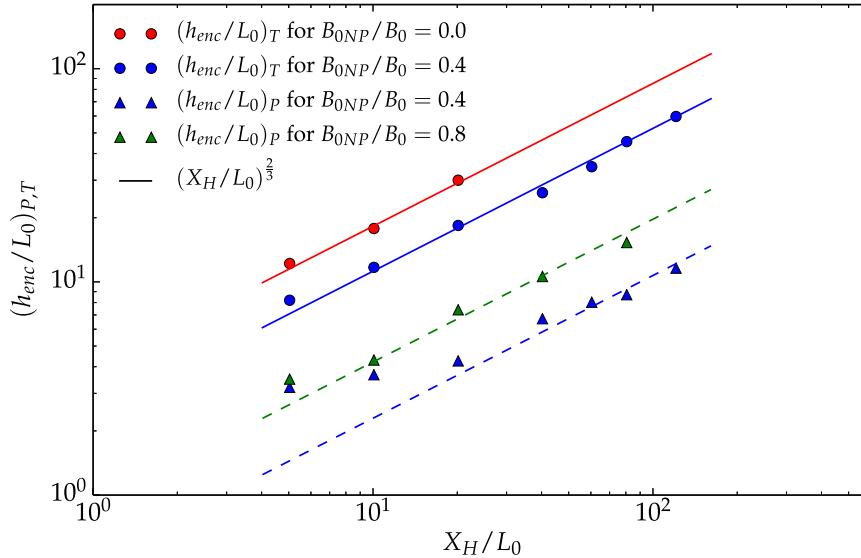
FIG. 10. Timings of the transitions  $(h_{enc}/X_H)_T$  and optimal states  $(h_{enc}/X_H)_P$  for the simulations in the first experiment (Table 1).
