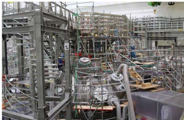
Fig. 2. Wendelstein 7-X in May 2014. On the left side, the so-called ‘‘Thomson bridge’’, which will support different diagnostics elements and allows access to the inner side of the torus is visible. On top of the device cable trays are mounted.
