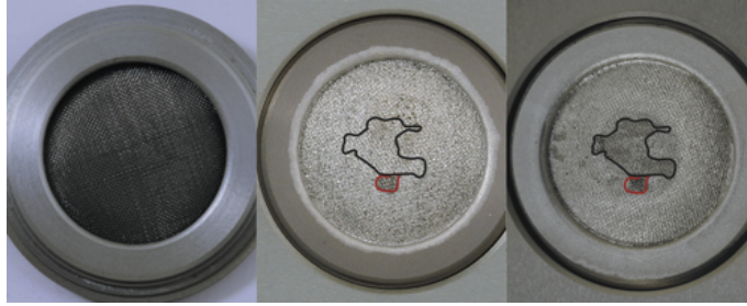
(a) CPS-like mesh strutter for PSI exposure, left to right: empty, before exposure, after exposure
