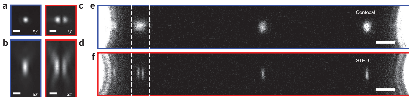
Figure 3 | Characterization of STED nanoscopy of proteins on optically stretched DNA. (a–d) Focal-intensity distributions of the 640-nm excitation (a,b) and 745-nm STED beam (c,d) imaged in the xy (a,c) and xz (b,d) planes. Scale bars, 500 nm. (e,f) Confocal microscopy (e) and subsequent STED image (f; power P_{\text{STED}} = 6 mW) of EcoRV–Atto 647N on \lambda DNA. Scale bars, 1 \mu\text{m} . (The ellipticity of the intensity
