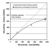
Figure 15: Binding capacity of the EEL membrane (3  $\mu$ m pore size, 75 cm<sup>2</sup>, 0.02 mg EEL/cm<sup>2</sup>): eluted viral product fraction (vertical axis, HA-activity) against loaded virus amount (horizontal axis, HA-activity,  $\Diamond$ : load below binding capacity, •: load above binding capacity)
