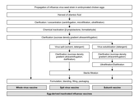
Figure 2: Example for the production procedure of egg-derived influenza virus vaccines
