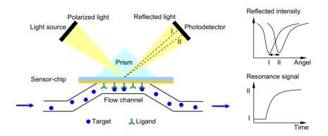
Figure 8: Schematic principle of interaction analysis by surface plasmon resonance technology (based on: Karlsson et al. 1991)
