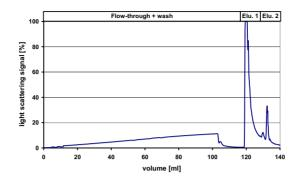
Figure 16: EEL-AC: human influenza virus A/Puerto Rico/8/34 capture from 100 ml unconcentrated cultivation broth by the EEL-polymer beads (3 ml column, 5.0 mg/ml ligand density; monitored by light scattering: 90°)
