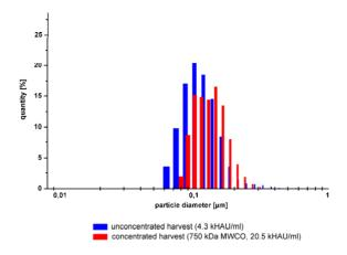
Figure 17: Particle-size-distribution analysis of concentrated (750 kDa MWCO) and unconcentrated cultivation broths containing influenza virus A/Puerto Rico/8/34
