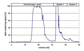
Figure 14: EEL-AC monitored by light scattering (90°): breakthrough of the EEL-membrane (3  $\mu$ m pore size, ligand density: 0.02 mg/cm<sup>2</sup>) loading human influenza A virus A/Puerto Rico/8/34 concentrate
