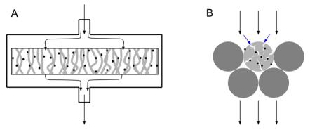
Figure 7: Schematic cross-section of a membrane layer (A) and chromatographic beads (B) (black dots: immobilized ligands; black arrows: flow direction of mobile phase; blue arrows: pore diffusion)
