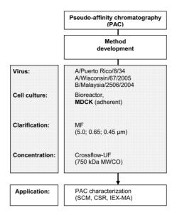
Figure 10: Overview about virus production used for PAC experiments (MF: microfiltration, UF: ultrafiltration)
