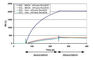
Figure 20: Comparative binding analysis of Vero- and MDCK cell-derived human influenza virus A/Puerto Rico/8/34 to EEL and ECL by SPR technology (Biacore 2000, association and dissociation phases are marked, signal changes due to sample matrix were eliminated by subtraction of the reference flow cell signal)
