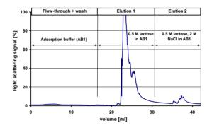
Figure 12: Light-scattering signal (90°) during purification of human influenza A virus concentrate with EEL-affinity chromatography (direct loading [0.2 ml/min] and elution [0.5 ml/min]; AB1: adsorption buffer 1)
