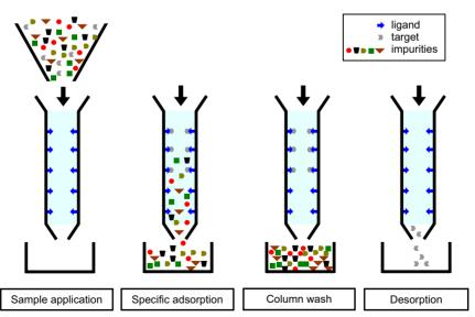
Figure 5: Principle of bead-based affinity chromatography
