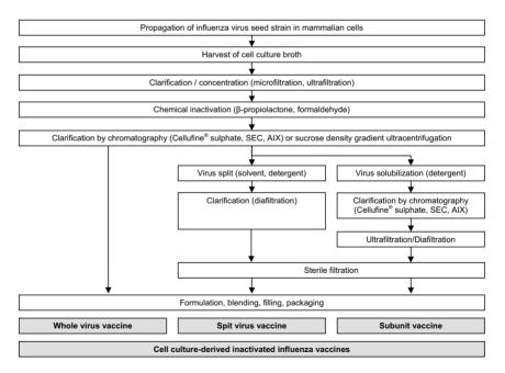
Figure 3: Example for the production procedure of cell culture-derived influenza virus vaccines
