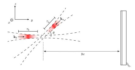
Fig. 1. The envisaged experimental set-up.  $\tau_{a,b}$  refer to the pulse durations in the Gaussian beam envelopes  $e^{-(t\pm y)^2/\tau_{a,b}^2}$ , the  $\mathbf{E}_b$  beam is displaced from the *y*-axis by co-ordinates  $x_0, z_0$ , both beams have in general a carrier-envelope phase and the  $\mathbf{E}_a$  beam lags behind  $\mathbf{E}_b$  by  $\Delta t$ . The  $\mathbf{E}_b$  field is incident on the detector.
