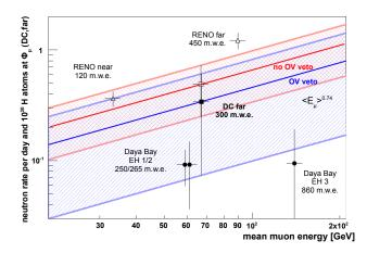
FIG. 2. Scaling of DC fast-n background rates and comparison with quoted values. Empty (full) markers indicate quoted results using a selection without (with) an external muon veto; lines and shaded bands represent our scaling of the DC measurements with their uncertainty. Values were scaled by number of H atoms and normalized to muon flux at DC far site.
