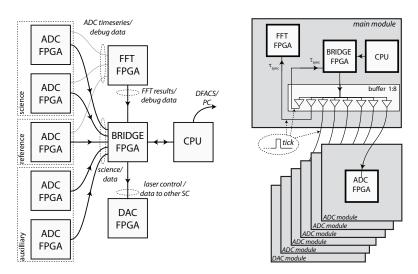
Figure 2. (left) System communication structure. All communication is routed through the bridge FPGA, with the exception of the highspeed data for the FFT FPGA. (right) Time tick distribution in the system via the bridge FPGA. All delays are matched, as well as the clock signals (not shown here), to allow a system wide hardware synchronization.
