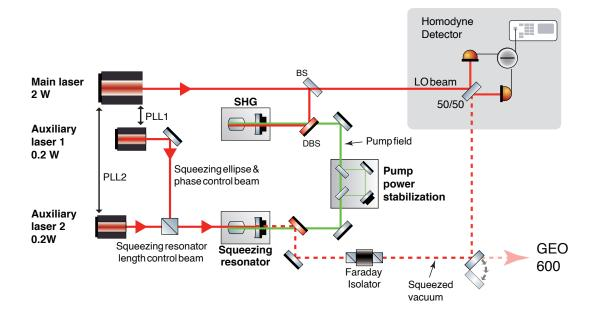
**Figure 1.** Simplified sketch of the optical layout of the squeezed-light laser. Auxiliary laser 1 is used to stabilize the length of the squeezing resonator and auxiliary laser 2 allows controlling the phase of the squeezed field. The two auxiliary lasers are phase locked (PLL) to the main 2W laser. For characterization, a balanced homodyne detector is available.
