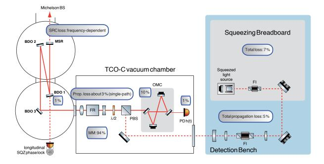
**Figure 3.** Sketch of the optical layout of the GEO 600 detection stage with squeezing input. Auxiliary optics are omitted for clarity reasons. The text boxes show estimations of the optical loss experienced by the squeezed field.
