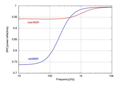
**Figure 4.** FINESSE simulation of the signal-recycling cavity's frequency-dependent power reflectivity with the old (blue trace) and new (red trace) MSR. The bandwidth of the SRC was increased from 220 Hz to 1100 Hz.
