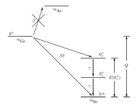
Figure 2: Scheme of the double beta decay of  $^{76}$ Ge. Single beta decay to  $^{76}$ As is energetically forbidden, thus the only open decay channel is double beta decay. It may proceed in the two-neutrino mode, as well as in the neutrinoless mode. Additionally, we will discuss the decay to the first excited  $0^+$  level.
