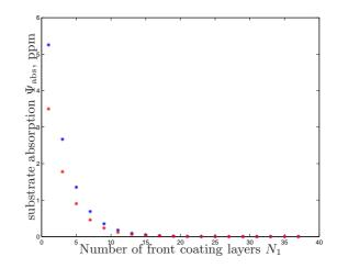
Figure 3: Substrate absorption  $\Psi_{abs}$  in ET (blue stars) and aLIGO (red stars) as a function of the number of front coating layers  $N_1$ . The number of rear coating layers  $N_2$  results from the total number of layers N = 38 minus the number of front layers  $N_1$ . Parameters used for this calculation are presented in Tables I and II.
