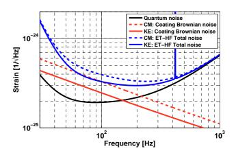
Figure 7: Potential overall sensitivity improvement of the ET high frequency detector (as described in [34]) for the use of KEs, compared to conventional end mirrors: The binary neutron star inspiral range increases by 15%, corresponding to a potential increase in the detected event rate for binary neutron star inspirals of 50%.
