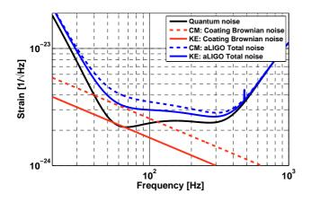
Figure 6: Potential overall sensitivity improvement of aLIGO for the use of KE, compared to conventional end mirrors: The binary neutron star inspiral range increases by 15% from 196.2 to 225.0 Mpc. This corresponds to a potential increase in the detected event rate for binary neutron star inspirals of slightly above 50%.
