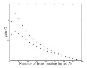
Figure 2: Gain G (see (14)) in ET (blue stars) and aLIGO (red stars) as a function of the number of front coating layers  $N_1$ . The number of rear coating layers  $N_2$  results from the total number of layers N = 38 minus the number of front layers  $N_1$ . Parameters used for this calculation are presented in Tables I and II. For ET a maximum gain of G = 1.72 appears for  $N_1 = 3$  front coating layers. For aLIGO the maximum gain of G = 2.16 is also obtained for  $N_1 = 3$ .
