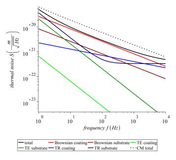
Figure 5: aLIGO noises spectral densities for KE with a front coating of  $N_1 = 5$  layers (plus a cap) and a rear coating of  $N_2 = 33$  layers (plus a cap). Parameters used for this calculation are presented in Table I and Table II.
