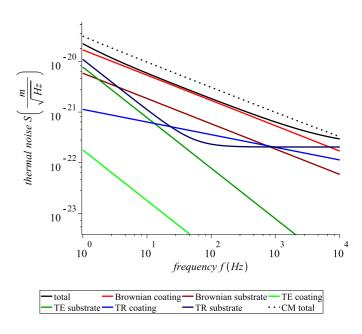
Figure 4: ET noise spectral densities for KE with a front coating of  $N_1 = 5$  layers (plus a cap) and a rear coating of  $N_2 = 33$  layers (plus a cap). Parameters used for this calculation are presented in Table I and Table II.
