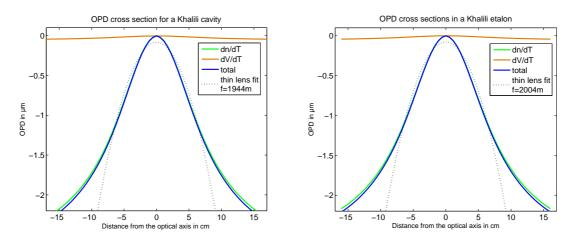
Figure 9: The optical path delay (OPD) is computed in the FEM simulation, in order to determine the focal length of the thermal lens in the KC (left) and the KE (right) for aLIGO parameters. Shown are the total OPD, the OPD caused by the thermo-refractive effect (named dn/dT) and the OPD due to the expansion of the substrate (dV/dT). The plots show also fits of the OPD for an ideal thin lens.
