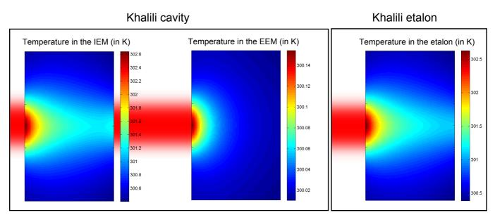
Figure 8: The temperature distribution in the mirrors of a KC (left) and a KE (right) for aLIGO parameters (with  $N_1=5$ ) as calculated via FEM. Please note the different color scales for the IEM and the EEM in the KC.
