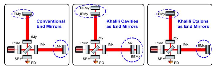
Figure 1: Simplified schematic of an Advanced LIGO interferometer with conventional end mirrors, featuring all the coating layers on their front (left), with Khalili cavities as end mirrors (center) and with Khalili etalons, featuring only a few coating layers on the front surface and the majority of the coating layers on the rear surface (right).
