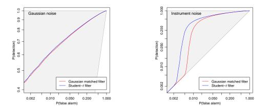
FIG. 4. ROC curves for the Gaussian and the Student-t detection statistics in both data scenarios. The shaded area marks the region where any sensible detection statistic (one that is not worse than mere guessing) should lie.
