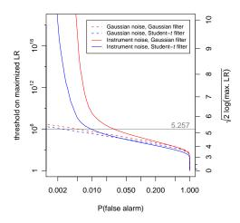
FIG. 5. Detection thresholds on the maximized likelihood ratio (the detection statistic), corresponding to certain false alarm probabilities. These thresholds are based on the detection statistic's distribution in the absence of a signal. The horizontal line indicates the injected signals' SNR (see also Fig. 4).
