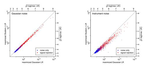
FIG. 3. Detection statistics (maximized likelihood ratios) based on Gaussian and Student-t models for simulated Gaussian data (left panel) and actual interferometer noise (right panel). Injections were of SNR  $\rho = 5.257$ .
